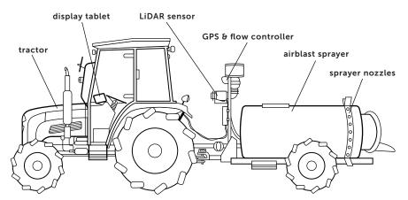
► LiDAR uses electromagnetic (EM) waves in the same way bats use sound waves to find their food. The system sends out these EM waves via laser pulses that bounce off objects and return to the sensor. The returning waves are interpreted into 3D images that display detailed information on objects in its surroundings. This 3D information tells the system exactly where and how much to spray.
