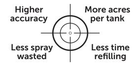
▶ Because it uses less spray volume per acre, the sprayer can spray more acres per tank of mixture, thus reducing tank refilling times.
