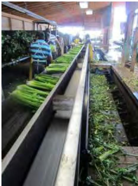
Figure 2. Conveying celery and removing trim
