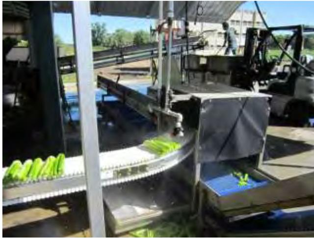
Figure 3. Celery cutting and spray washing/sanitizing
